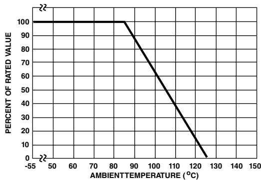
Figure 1A - Power Derating for Epoxy Coated
