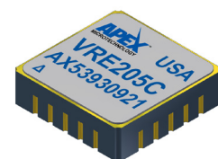
20-terminal Ceramic LCC Package Style HD
