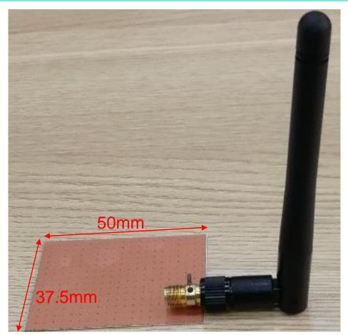
Test with a 37.5mm\*50mm ground plane in free space.
