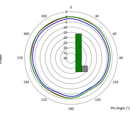
Avg -3(deg) = 339.5 433MHz Avg (dBi) = -1.55 Peak (dBi) = -0.08 Avg -3 (deg) = 333.5 435MHz Avg (dBi) = -1.38 Peak (dBi) = 0.13 Avg -3 (deg) = 328.5
