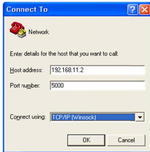
Figure 18. Network Terminal Program configuration
