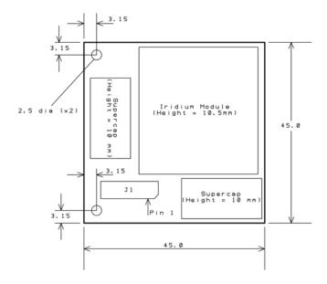
\*Note that the diagram and dimensions do not include the SMA connector
