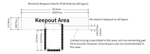
Recommended Keepout Area for PCB Antenna (All layers)
