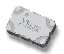
The X3C07F1-05S is a low profile, high performance 5dB directional coupler in a new easy to use, manufacturing friendly surface mount package. It is designed for DCS, UMTS, LTE and PCS applications. The X3C07F1-05S is designed particularly for non-binary split and combine in high power amplifiers, e.g. used along with a 3dB to get a 3-way, plus other signal distribution applications where low insertion loss is required. It can be used in high power applications up to 25 Watts.
