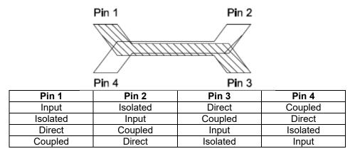
Note: The direct port has a DC connection to the input port and the coupled port has a DC connection to the isolated port.
