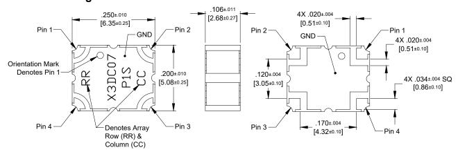
Dimensions are in Inches [Millimeters] X3DC07P1S Mechanical Outline
