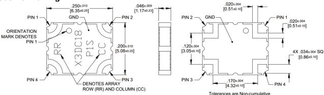
Dimensions are in Inches [Millimeters] X3DC18P1S Mechanical Outline
