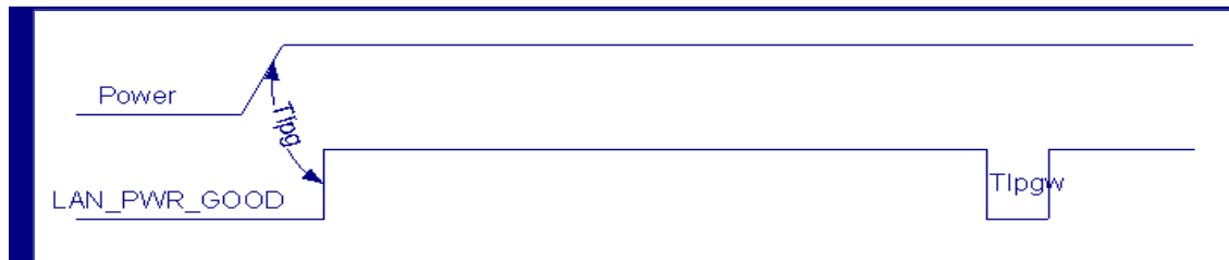
Figure 12-7. External Reset Timing Diagram
