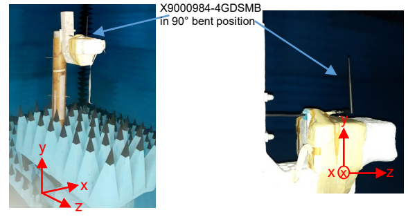
Antenna measured in Free Space
