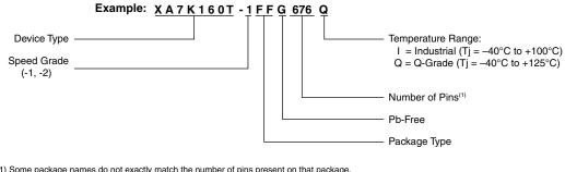
Some package names do not exactly match the number of pins present on that package. See UG475, 7 Series FPGAs Packaging and Pinout User Guide for package details.
