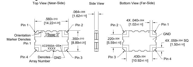
Dimensions are in Inches [Millimeters] XC0900A-05\* Mechanical Outline
