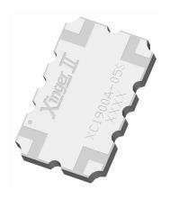
The XC1900A-05 is a low profile, high performance 5dB directional coupler in a new easy to use, manufacturing friendly surface mount package. It is designed for DCS and PCS applications. The XC1900A-05 is designed particularly for non-binary split and combine in high power amplifiers, e.g. used along with a 3dB to get a 3-way, plus other signal distribution applications where low insertion loss is required. It can be used in high power applications up to 200 Watts.
