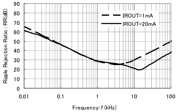
XC6408D/E ( V_{ROUT}=12.0V , V_{IN}=14.0V_{DC}+0.5V_{p-pAC} ) ( C_L=1.0\mu F (Ceramic), T_a=25^\circ C )
