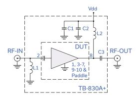
Fig 1. Application and Characterization Circuit
