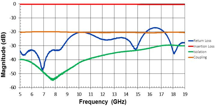
\*Typical measured performance mounted on RO4350B test board at 25°C.
