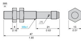
(1) LED, 4 viewing ports at 90° Note Fixing nut tightening torque : <2N.m
