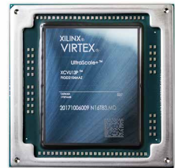
Xilinx VU13P FPGA: lidless package is used by BittWare's Viper thermal management for enhanced cooling performance
