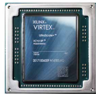
Xilinx VU13P FPGA: lidless package is used by BittWare's Viper thermal management for enhanced cooling performance
