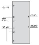
With External Device Monitoring (EDM) feedback loop
