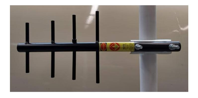
Antenna mounted vertically on post with insulator on driven element facing up
