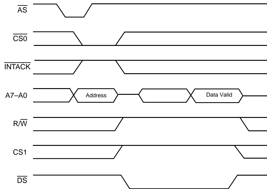
Figure 18. Z80230 Read Cycle Timing
