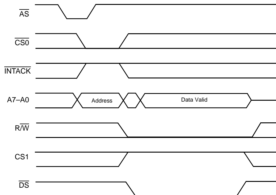
Figure 17. Z80230 Write Cycle Timing
