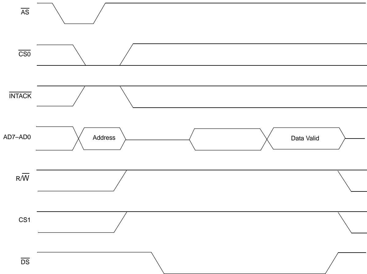
Figure 24. Read Cycle Timing
