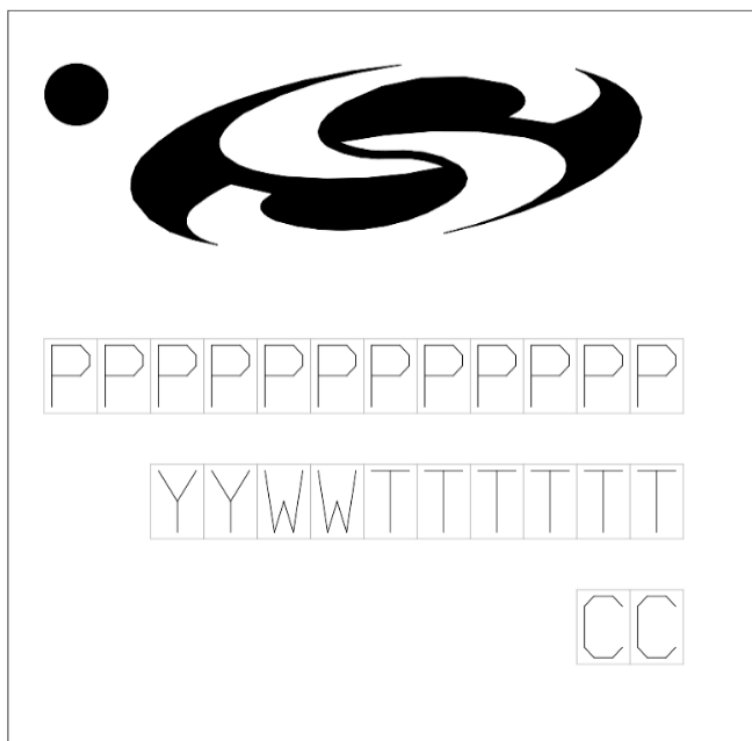
Figure 7.3. LGA64 Package Marking
