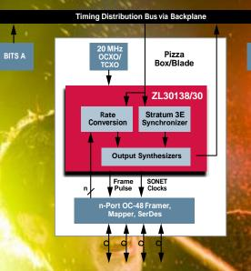
**Centralized System Timing And Blade Applications**
