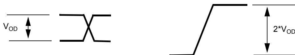
Figure 19 - Differential Voltage Parameter
