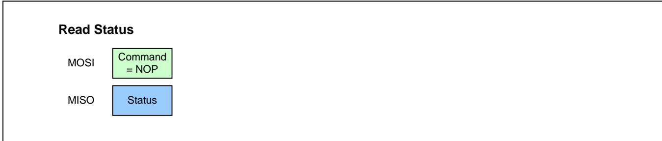
Figure 3.6 SPI Read Status
