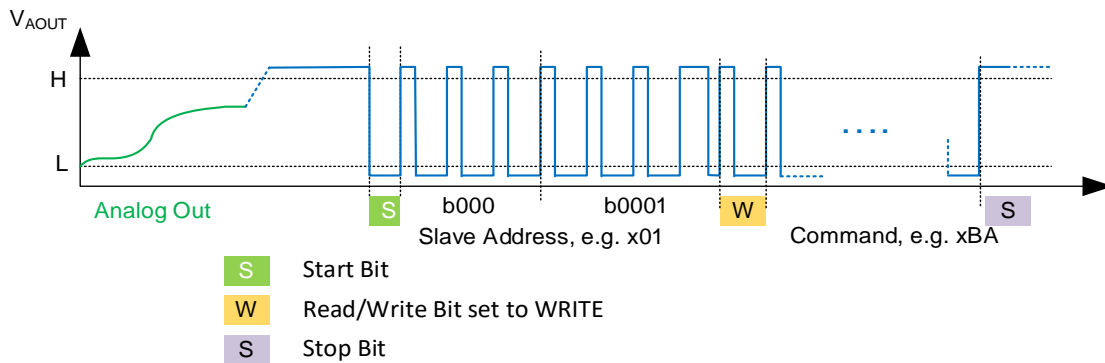
Figure 54: Typical OWI Communication on AOUT in Voltage Out Mode
