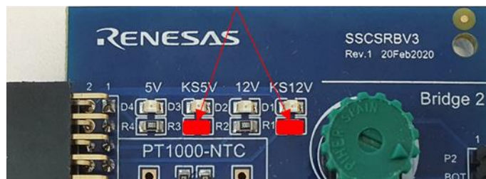
Figure 129. 2-Wire Current Loop SRB3 Specific Configuration
