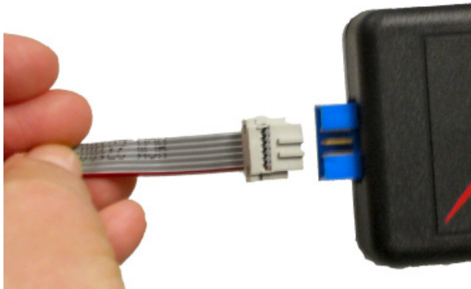
Figure 1. Connecting the Six-Conductor Ribbon Cable to the Acclaim! Smart Cable
