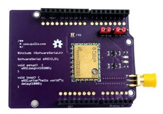
This 'shield' allows Arduino™ boards to communicate wirelessly using proprietary LPRS 'easyRadio' technology operating in the 433MHz or 868/915MHz (Industrial Scientific & Medical (ISM) bands.
