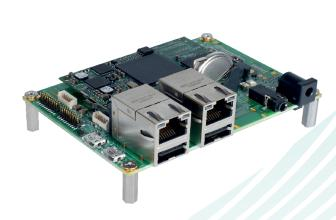
iWave's i.MX6 SODIMM development board incorporates i.MX6 SODIMM SOM Which is based on Freescale's high performance i.MX6 Quad ARM Cortex A9 processor and the carrier board with optional 4.3" resistive display kit. The development board can be used for quick prototyping of various applications targeted by the i.MX6 processors. With the 100mm x72 mm Pico ITX size, the kit is highly packed with all the necessary on-board connectors to validate the i.MX6 CPU features.
