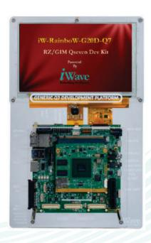
iWave's RZ/G1M development board incorporates RZ/G1M QSeven SOM which is based on Renesas high performance RZ/G1M Dual ARM Cortex A15 MPU and the carrier board with optional 7" capacitive Display Kit. The development board can be used for quick prototyping of various applications targeted by the RZ/G1M processor. With the 120mm x 120mm Nano ITX size, the kit is highly packed with all the necessary on-board connectors to validate the RZ/G1M MPU features.
