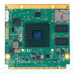
iWave's RZ/G1-M based Qseven CPU module integrates high performance ARM Cortex A15 Dual CPU core operating up to 1.5GHz speed. The SOM is packed with rich set of features and IO peripherals. It integrates HD Hardware codecs, graphic acceleration, on-board PMIC, eMMC flash, DDR3 RAM, Micro SD slot, USB Hub and Gigabit Ethernet PHY. The SOM is ideally suitable for high performance general embedded, industrial and video intensive applications.
