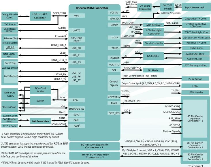
5 VI1 & VI2 can be used in 8bit mode. If VI1 is used in 16bit, then VI2 cannot be used.
