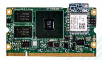
iWave's RZ/G1E based SODIMM system on module integrates power efficient ARM Cortex A7 Dual core CPU operating up to 1GHz speed and with 802.11n Wi-Fi & BLE4.0 Module. The SOM is packed with rich set of features and IO peripherals. It integrates HD hardware codecs, 3D Graphics Acceleration, DDR3 RAM, eMMC Flash, Gigabit and 10/100 Ethernet PHY. The SOM is ideally suitable for low power, cost effective, general embedded, industrial and video intensive applications.
