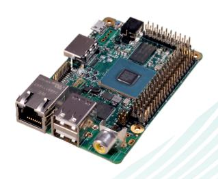
iWave's RZ/G1C SBC is based on Renesas power efficient Dual/Solo core ARM Cortex A7 CPU cores operating @1GHz speed. This board can be used for quick prototyping of various applications targeted by the RZ/G1C processor. With the 85mm x 56mm size, the kit is highly packed with all the necessary on-board connectors to validate the RZ/G1C CPU features.
