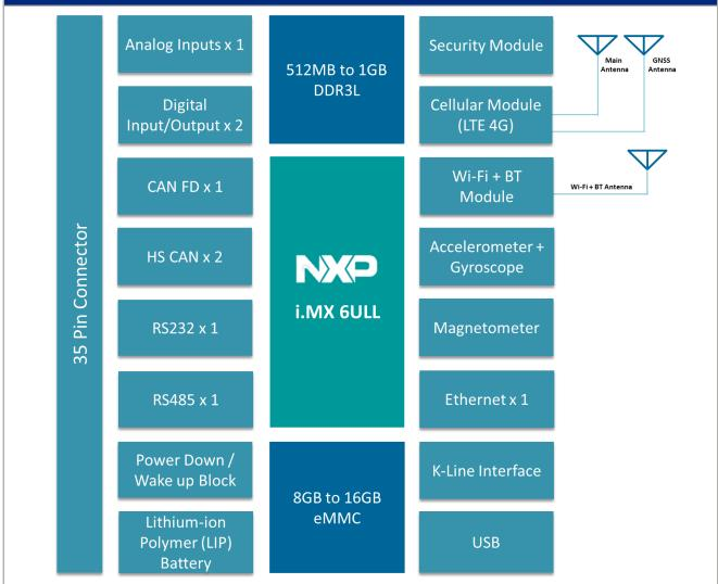
Note: Standard delivery varies with respect to the few sections of this block diagram, depending on the ordered configuration
