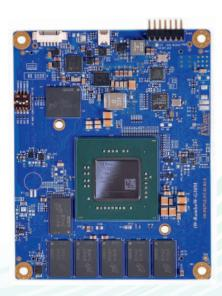
Xilinx Zynq UltraScale+ SoC based System On Module features the Xilinx's Zynq UltraScale+ SoC CG/EG/EV devices with B900 package. The MPSoC supports Quad/Dual Cortex A53 up to 1.5GHz with programmable logic cells ranging from 192K to 504K. The SOM supports high speed connectivity peripherals such as PCle, USB3.0, SATA3.1, Display port, Gigabit Ethernet through GTR high speed transceivers from MPSoC.
