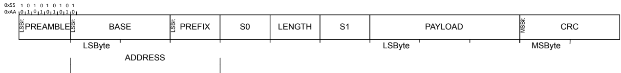
Figure 136: On-air packet layout
