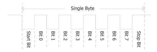
uLCD-90D Series Serial Ports - TTL Level
