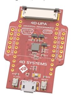
The 4D-UPA is a single module with a micro USB interface, and DIP-style pads for GPIO breakout of all the signals used on the Display interface, which is useful for development or final product use. Standard 2.54mm (0.1") male pin headers can be mounted so the module signals can be interfaced to easily.
