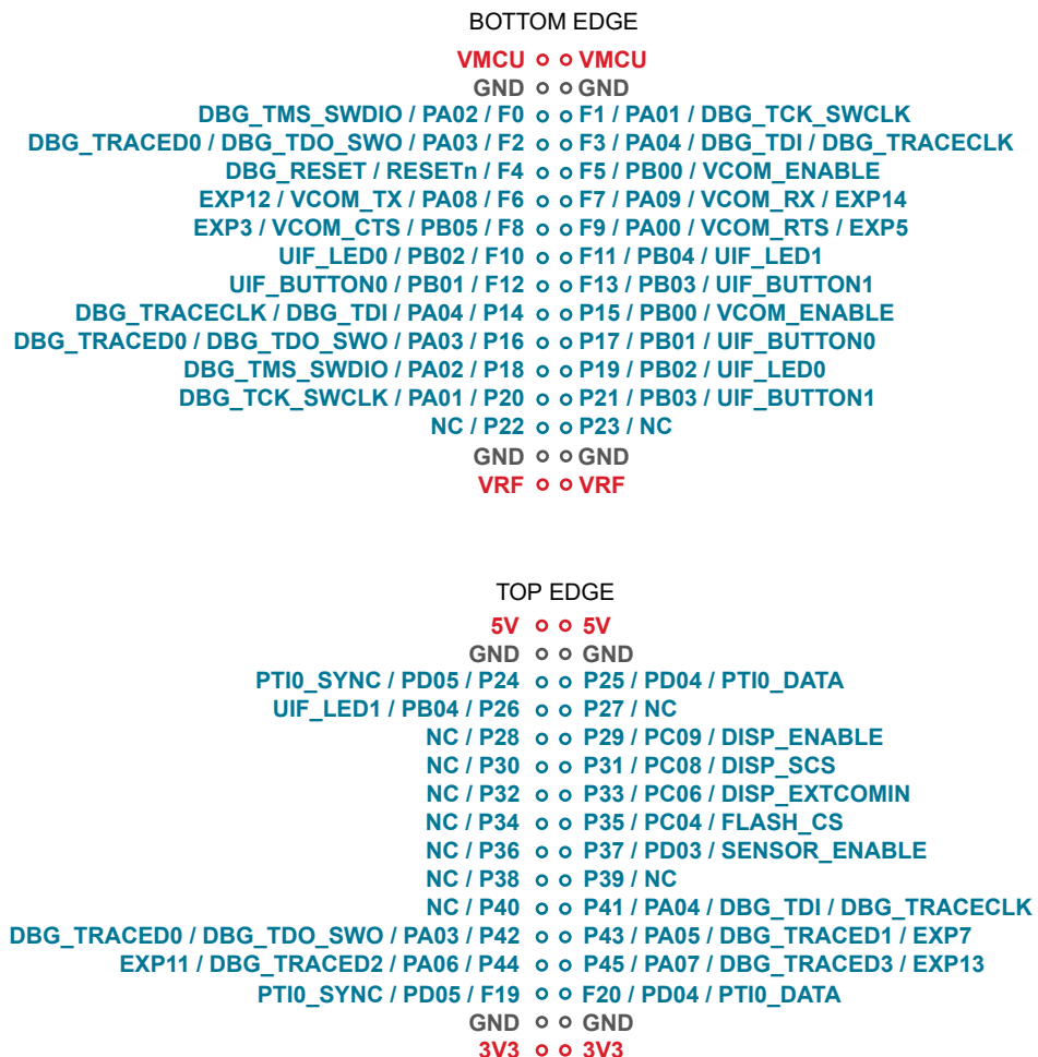
Figure 3.3. Wireless Pro Kit Mainboard (BRD4002A) Breakout Pad Pin Mapping
