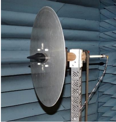
antenna sample measured on \varnothing 24'' (609.6mm) ground plane
