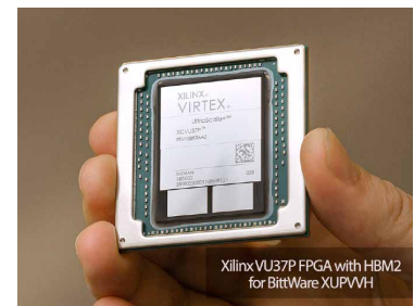
Xilinx VU37P FPGA: lidless package is used by BittWare's Viper thermal management for enhanced cooling performance
